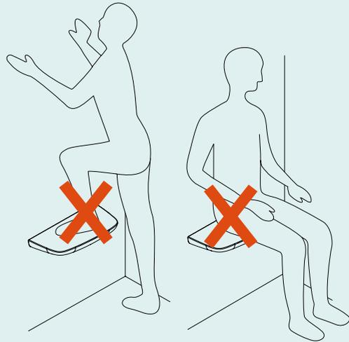
**Please note:** Due to safety reasons, Corniche should only be installed by a professional. The specified max. load only applies if Corniche has been installed correctly taking the wall structure into consideration. The mounting materials are suitable for walls made of concrete or brick, but not for hollow walls.
